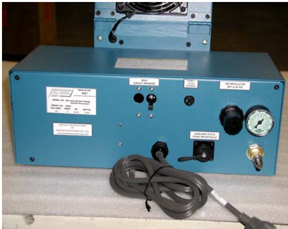
M425 rear panel with circuit breaker, air regulator, air connection and foot switch port
